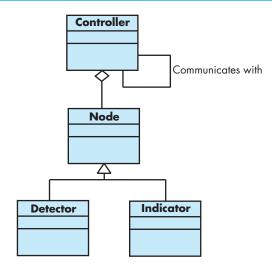
Each of these archetypes is depicted using UML notation as shown in Figure 13.7. Recall that the archetypes form the basis for the architecture but are abstractions that must be further refined as architectural design proceeds. For example, **Detector** might be refined into a class hierarchy of sensors.
