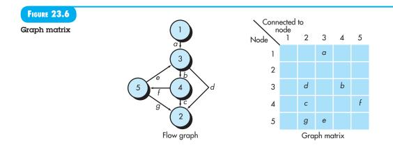
matrix can become a powerful tool for evaluating program control structure during testing. The link weight provides additional information about control flow. In its simplest form, the link weight is 1 (a connection exists) or 0 (a connection does not exist). But link weights can be assigned other, more interesting properties:
