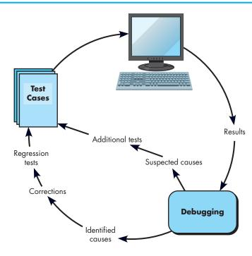
Results are assessed and a lack of correspondence between expected and actual performance is encountered. In many cases, the noncorresponding data are a symptom of an underlying cause as yet hidden. The debugging process attempts to match symptom with cause, thereby leading to error correction.
