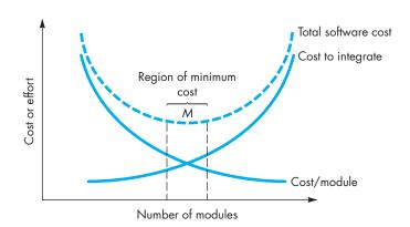
modules increases. Given the same set of requirements, more modules means smaller individual size. However, as the number of modules grows, the effort (cost) associated with integrating the modules also grows. These characteristics lead to a total cost or effort curve shown in the figure. There is a number, M, of modules that would result in minimum development cost, but we do not have the necessary sophistication to predict M with assurance.
