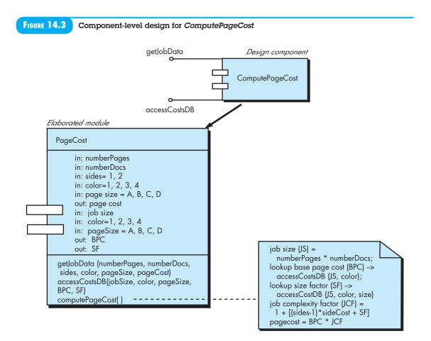
a collection of input and output data objects or items. Design elaboration continues until sufficient detail is provided to guide construction of the component.
