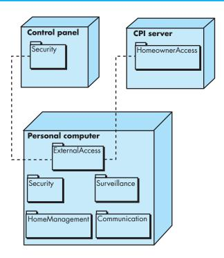
identified. It could be a Mac, a Windows-based PC, a Linux-box or a mobile platform with its associated operating system. These details are provided when the deployment diagram is revisited in *instance form* during the latter stages of design or as construction begins. Each instance of the deployment (a specific, named hardware configuration) is identified.
