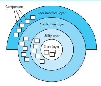
**Object-Oriented Architectures.** The components of a system encapsulate data and the operations that must be applied to manipulate the data. Communication and coordination between components are accomplished via message passing.
