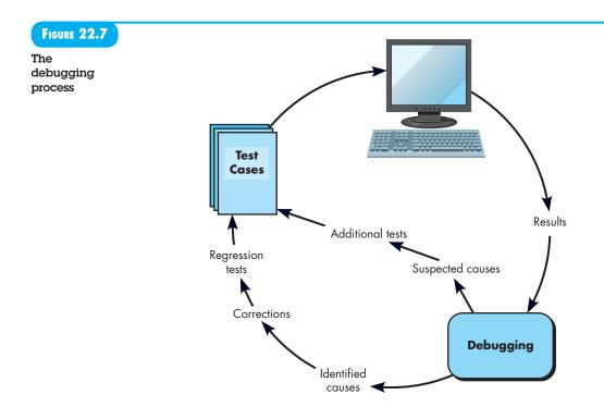
Results are assessed and a lack of correspondence between expected and actual performance is encountered. In many cases, the noncorresponding data are a symptom of an underlying cause as yet hidden. The debugging process attempts to match symptom with cause, thereby leading to error correction.
