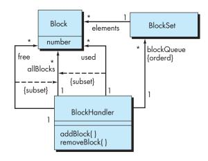
Note that each expression starts with the keyword *context*. This indicates the element of the UML diagram that the expression constrains. The keyword **self** here refers to the instance of **BlockHandler**; in the following, as is permissible in OCL, we will omit the **self**.
