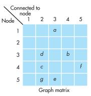
matrix can become a powerful tool for evaluating program control structure during testing. The link weight provides additional information about control flow. In its simplest form, the link weight is 1 (a connection exists) or 0 (a connection does not exist). But link weights can be assigned other, more interesting properties:
