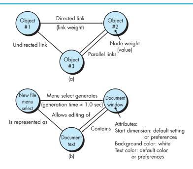
have the expected relationship to one another" [Bei95]. Stated in another way, software testing begins by creating a graph of important objects and their relationships and then devising a series of tests that will cover the graph so that each object and relationship is exercised and errors are uncovered.
