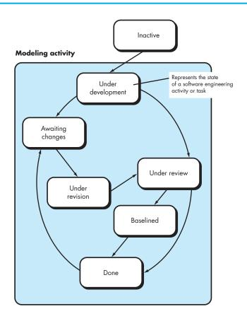
model is uncovered. This generates the event *analysis model correction*, which will trigger the requirements analysis action from the **done** state into the **awaiting changes** state.
