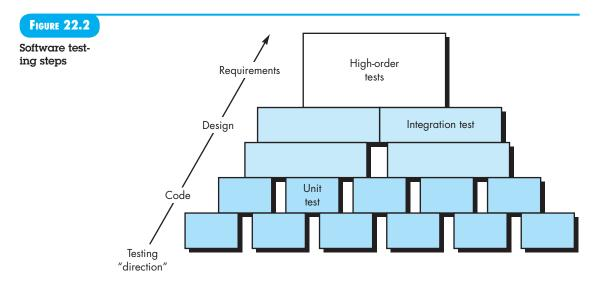
The last high-order testing step falls outside the boundary of software engineering and into the broader context of computer system engineering. Software, once validated, must be combined with other system elements (e.g., hardware, people, databases). *System testing* verifies that all elements mesh properly and that overall system function/performance is achieved.
