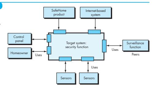
As part of the architectural design, the details of each interface shown in Figure 13.6 would have to be specified. All data that flow into and out of the target system must be identified at this stage.
