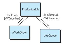
messages that are passed between objects within a system. Although this design activity is optional, it can be used as a precursor to the specification of interfaces that show how components within the system communicate and collaborate.
