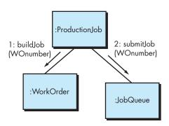
messages that are passed between objects within a system. Although this design activity is optional, it can be used as a precursor to the specification of interfaces that show how components within the system communicate and collaborate.
