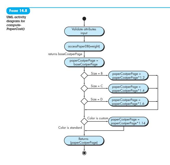
**Step 5. Develop and elaborate behavioral representations for a class or component.** UML state diagrams were used as part of the requirements model to represent the externally observable behavior of the system and the more localized behavior of individual analysis classes. During component-level design, it is sometimes necessary to model the behavior of a design class.
