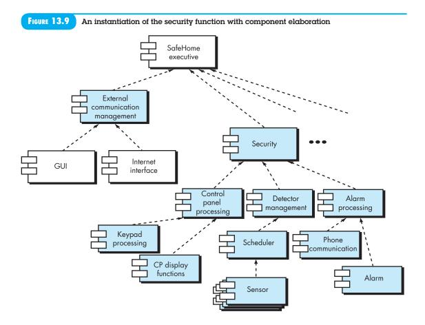
a *scheduler* infrastructure component that implements polling of each *sensor* object used by the security system. Similar elaboration is performed for each of the components represented in Figure 13.8.
