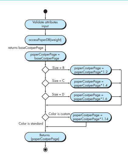
Step 5. Develop and elaborate behavioral representations for a class or component. UML state diagrams were used as part of the requirements model to represent the externally observable behavior of the system and the more localized behavior of individual analysis classes. During component-level design, it is sometimes necessary to model the behavior of a design class.
