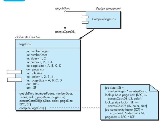
a collection of input and output data objects or items. Design elaboration continues until sufficient detail is provided to guide construction of the component.
