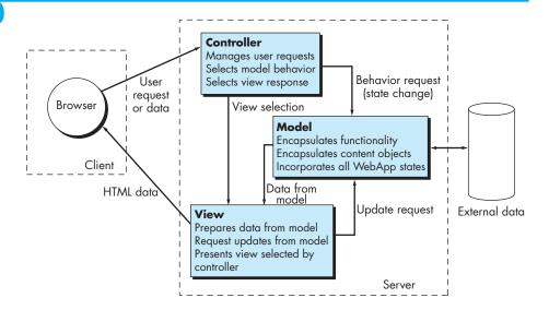
a corporate database, as part of a local data store, or as a collection of independent files. The data developed by the model must be formatted and organized by the appropriate view object and then transmitted from the application server back to the client-based browser for display on the customer's machine.
