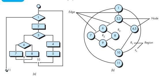
introduced.<sup>3</sup> The flow graph depicts logical control flow using the notation illustrated in Figure 23.1. Each structured construct (Chapter 14) has a corresponding flow graph symbol.
