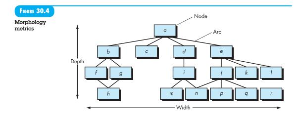
The arc-to-node ratio, r = a/n, measures the connectivity density of the architecture and may provide a simple indication of the coupling of the architecture. For the architecture shown in Figure 30.4, r = 18/17 = 1.06.
