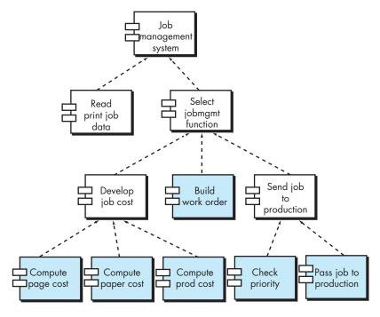
Control components (modules) reside near the top of the hierarchy (program architecture), and problem domain components tend to reside toward the bottom of the hierarchy. To achieve effective modularity, design concepts like functional independence (Chapter 12) are applied as components are elaborated.
