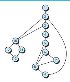
without developing a flow graph by counting all conditional statements in the PDL (for the procedure *average*, compound conditions count as two) and adding 1. Referring to Figure 23.5,
